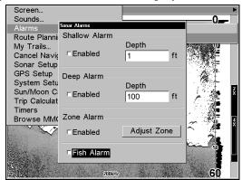
Sonar Alarms menu with Fish Alarm selected. The checkbox is blank, indicating the alarm is turned off.
